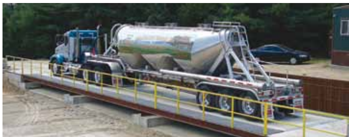
Facility inbound/outbound vehicle weighing using a single truck scale
